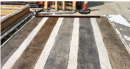
Color samples for sealants for the new bridge deck. Photos courtesy of Lincoln Parks and Recreation
